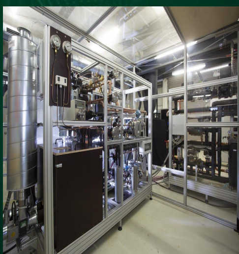
© Fraunhofer ISE Test-rig for the measurement of heat exchangers exposed to refrigerant (evaporators and condensers)(Pic Ref: https://www.ise.fraunhofer.de/en/research-projects/owex-bestand-htwp.html )
